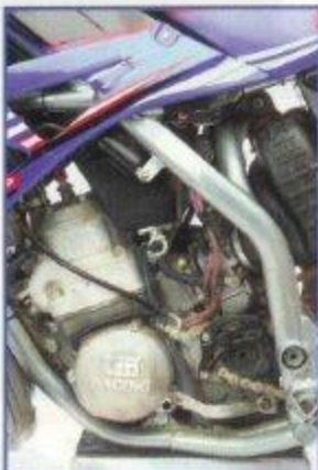
Silver oval: The Italian frame is innovative. Its semi-perimeter design uses ovalized chromoly tubes to cocoon the case-reef engine. It looks trick, but is on the heavy side.
